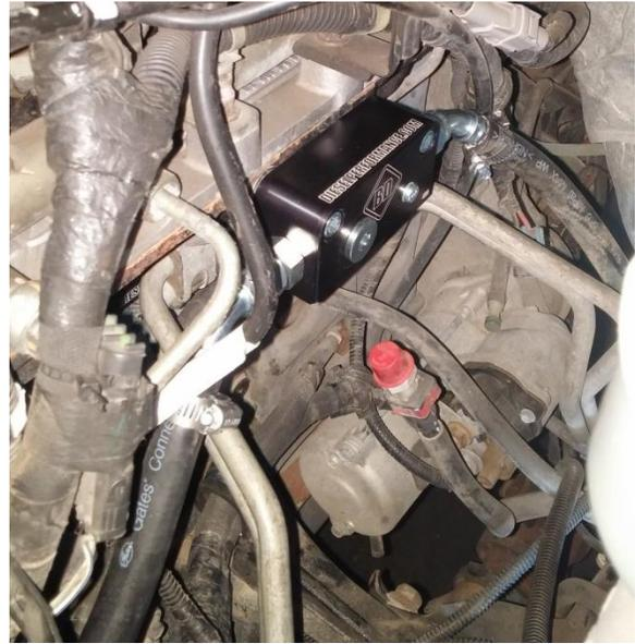
22. The connections for the factory WIF sensor and fuel heater will now be exposed. It is highly recommended that a WIF extension harness be installed into the factory connector to allow the use of an auxiliary WIF sensor.
