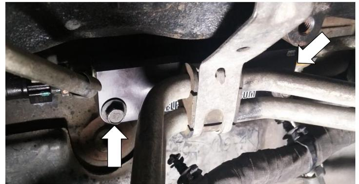
16. Slide a seal washer between the fuel block and return line, and install the original banjo bolt with the new washers.
