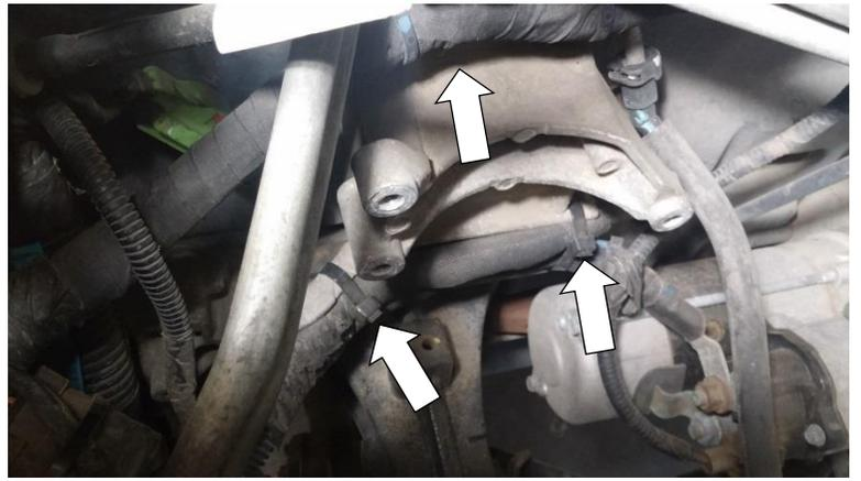
7. Remove the return quick-connect and remove the banjo bolts from the fuel return bracket with a 17mm socket. Set these aside, as they will be re-used later for install.
