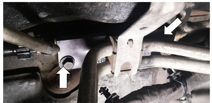
18. Using the supplied insulated loop clamp, and bolt. Secure the starter cables to the top of the motor mount.
