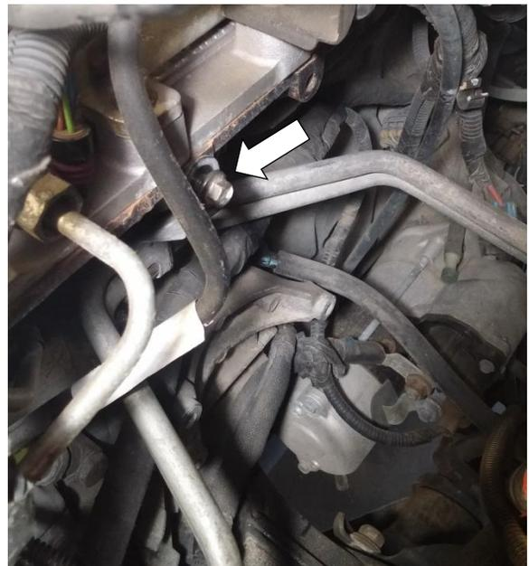
9. Remove the three (3) screws holding the bracket to the engine using a 10mm socket. Remove bracket from engine.
