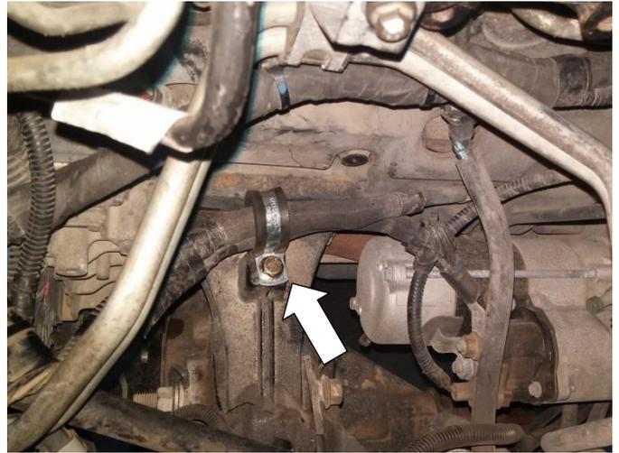
19. Install the assembled feed distribution block to the empty threaded holes on the side of the cylinder head, using the supplied M8 fasteners. Torque fasteners to **24 Ft-lbs** using 6mm hex bit
