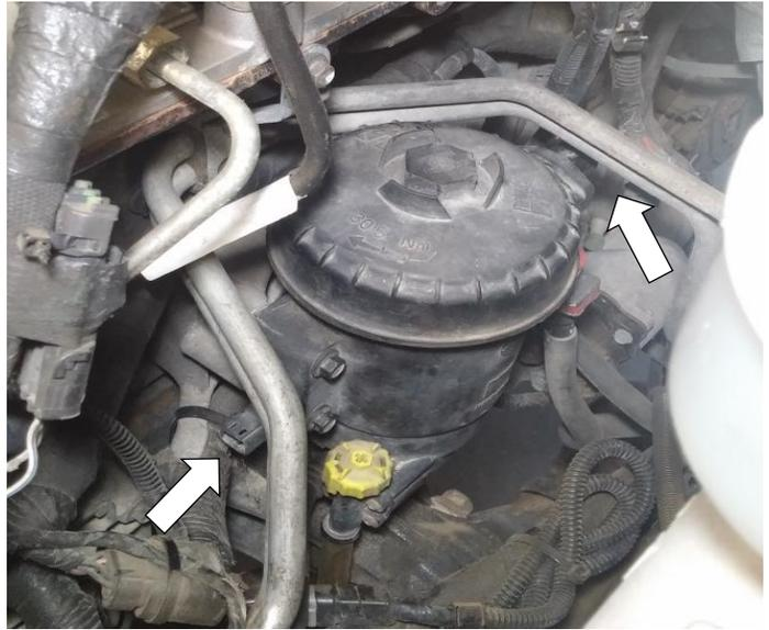
4. Disconnect the factory fuel quick connects from the fuel bowl, if still in use. (Fuel bowl shown removed for clarity)
