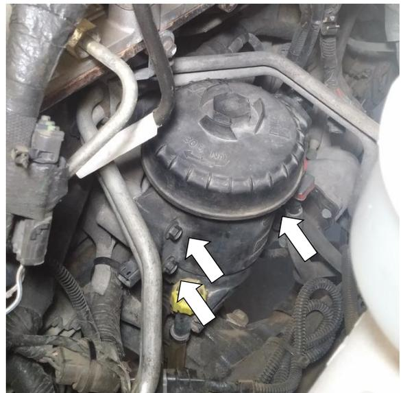
6. Cut zip-ties holding battery cables, and pull the upper wiring harness off the fuel bowl bracket.
