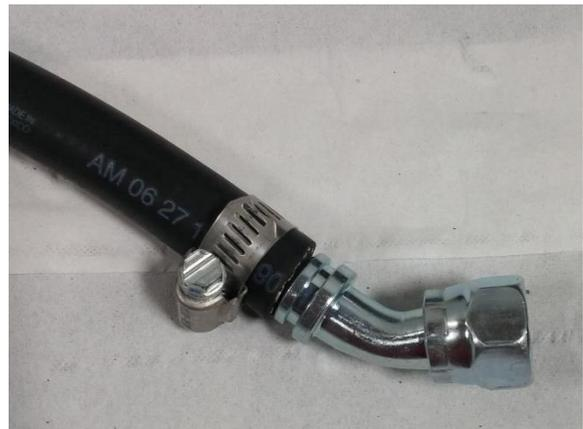
21. Ensure all fittings are tight, and hoses are zip tied away from any hot or moving parts in the engine bay.
