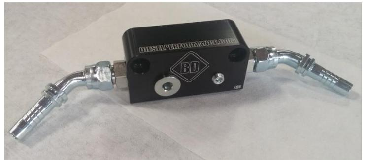
13. Shown is the return block with the -6 plug being installed.
