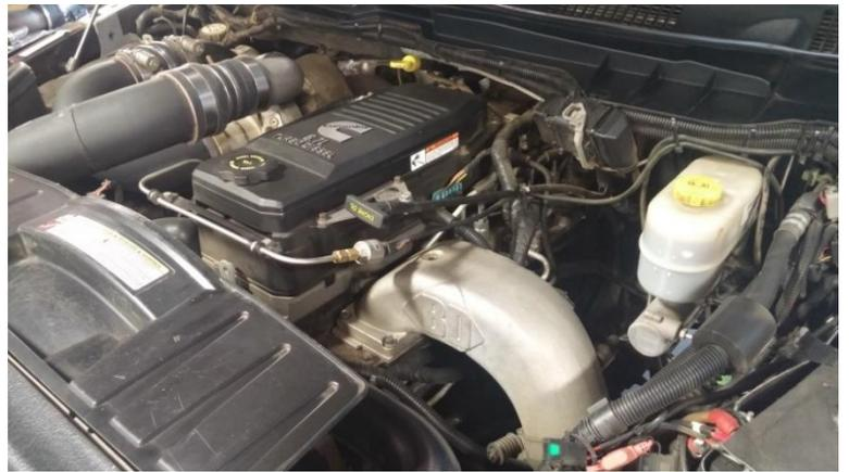
2. Place a pan or bucket below the fuel bowl and drain as much fuel out as possible by turning the drain valve. This will help reduce fuel spill when the fuel lines are disconnected.
