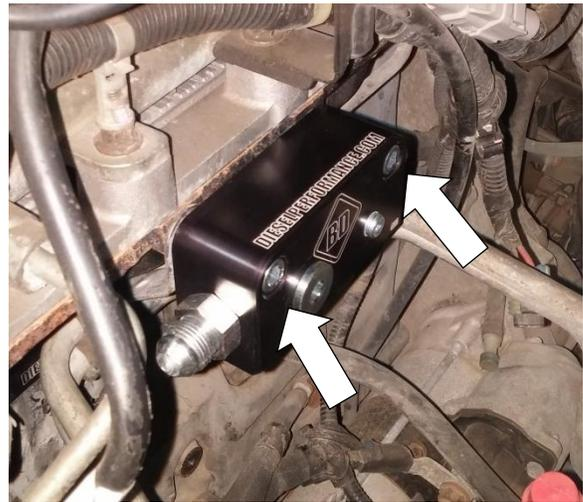
20. If running the fuel feed through the distribution block, attach the supplied swept -8 JIC to a 1/2" fuel hose (not supplied), and connect the hoses to their respective fittings.
