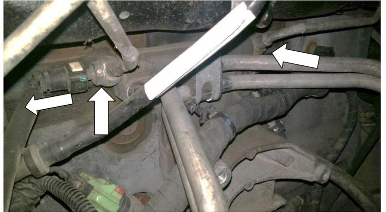
8. If you have a 2010-12 model year truck, you may have to remove the bolt holding the transmission lines in place to gain clearance for bracket access.
