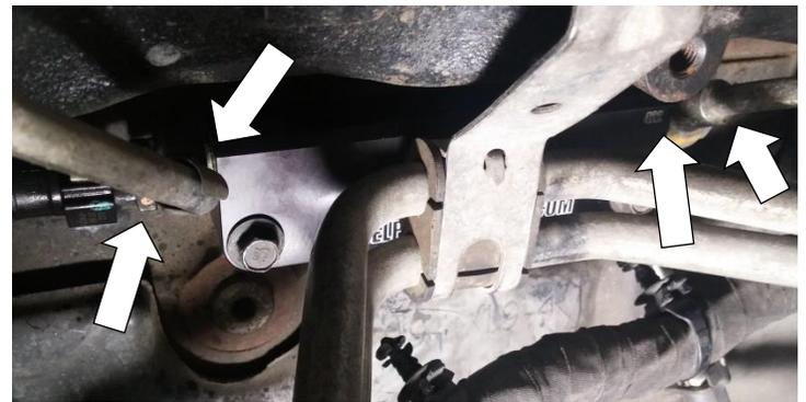
17. Tighten the two bolts holding the fuel distribution block to the engine block using a 10mm socket to **24 Ft-lbs.**
